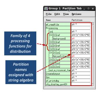
Figure 5 - Example of function partitioning table used to specifiy implementation
