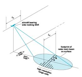
Figure 1 - Geometry of Example RADAR
